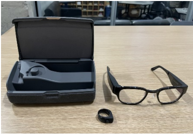
Figure 1: Focals by North version 1.0 with glasses, carrying charger case, and Loop (ring toggle for index finger).
